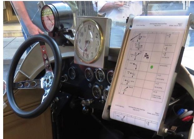
A sophisticated setup for a GR car, with race instructions, an expensive clock with a sweep hand, and a super-accurate $1000 speedometer
